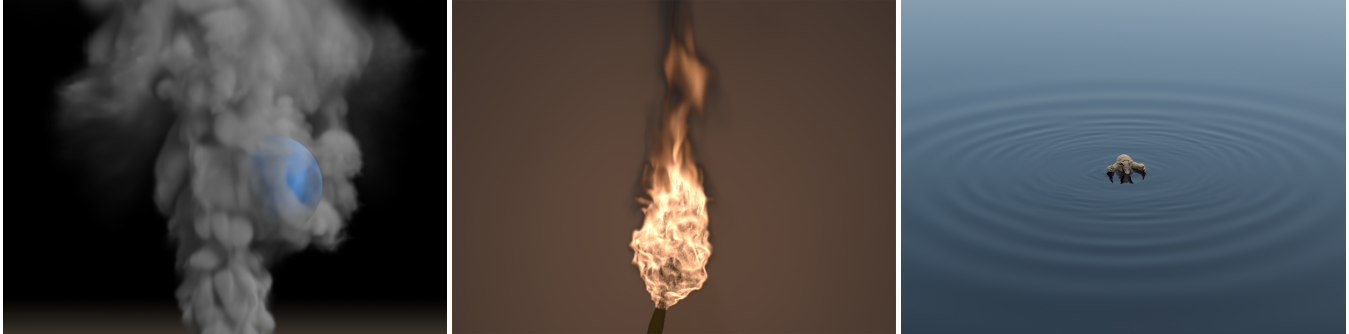
Figure 1: Our far-field grid structure provides an extended domain for fluid simulations of smoke, fire, and water. (Left) A fine grid follows the sphere in order to resolve the fine scale details of the smoke due to object interaction while the extended grid allows the smoke to rise until it is off camera – see Figure 5. (Center) A torch that moves through a large extent of the domain uses a fine grid to track the torch motion while grid extension allows for larger camera angles – see Figure 6. (Right) A large advantage of our extended grid is that it allows outgoing waves to avoid reflecting off of grid boundaries thus allowing for a large amount of detail and grid resolution near the region of interest without reflected waves.
